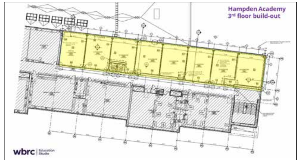
Floor plan shows eight new classrooms from third-floor buildout at Hampden Academy.
